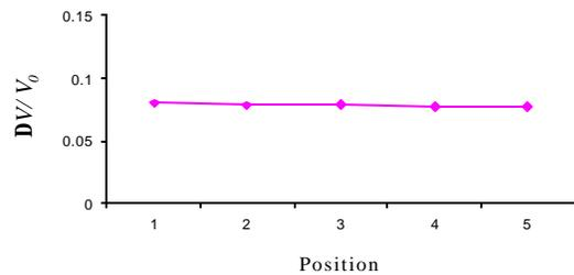
(c) Relative output change of shear stress sensors
