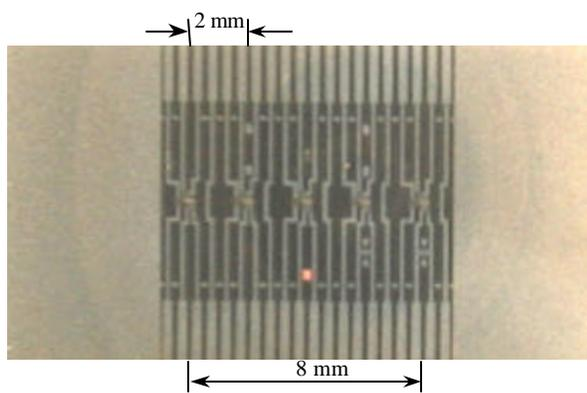
(b) Picture of a multi-sensor array chip.
