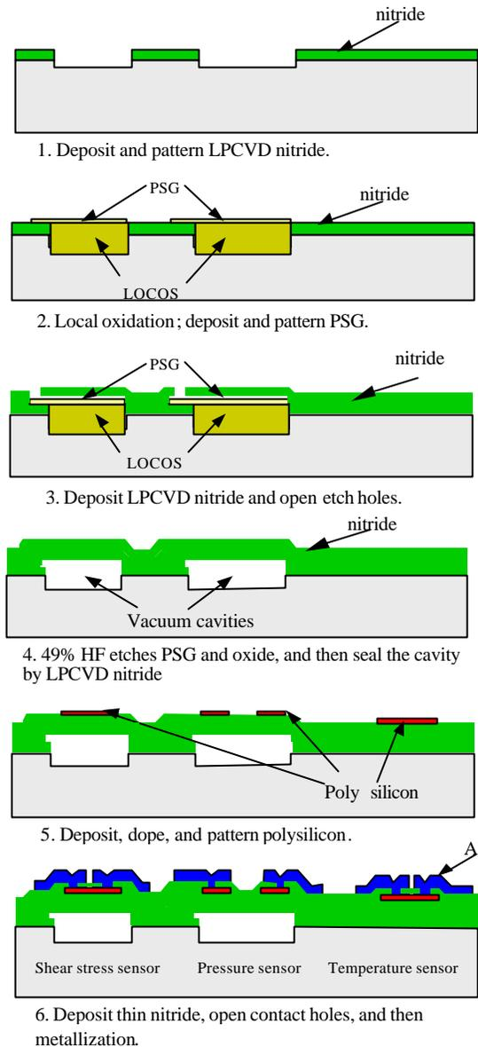
Figure 1 Simplified fabrication process.
