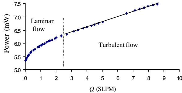
Figure 8 Response of shear stress sensor ( $h=200\ \mu\text{m}$ ,  $a_R = 10\%$  and  $\text{N}_2$  flow).
