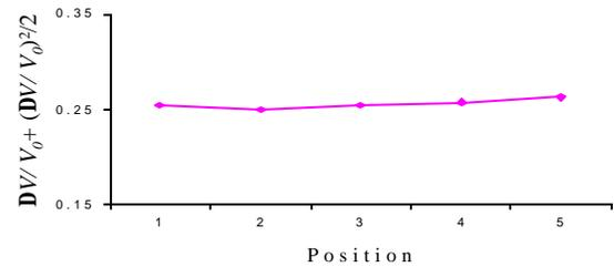
(c) Relative output change of shear stress sensor
