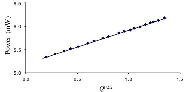
Figure 9 Input power versus  $Q^{1/2.2}$  (laminar flow region).
