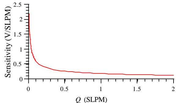
Figure 10 Sensitivity of the thermal flowmeter in laminar flow regime
