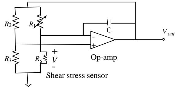
Figure 4 Simplified constant temperature bias circuit.
