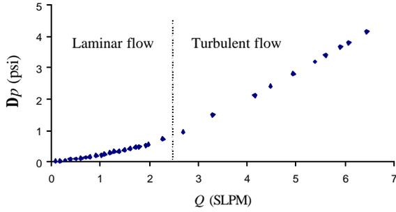
Figure 7 Pressure drop vs. mass flow rate ( $h=200\ \mu\text{m}$  and  $\text{N}_2$  flow).
