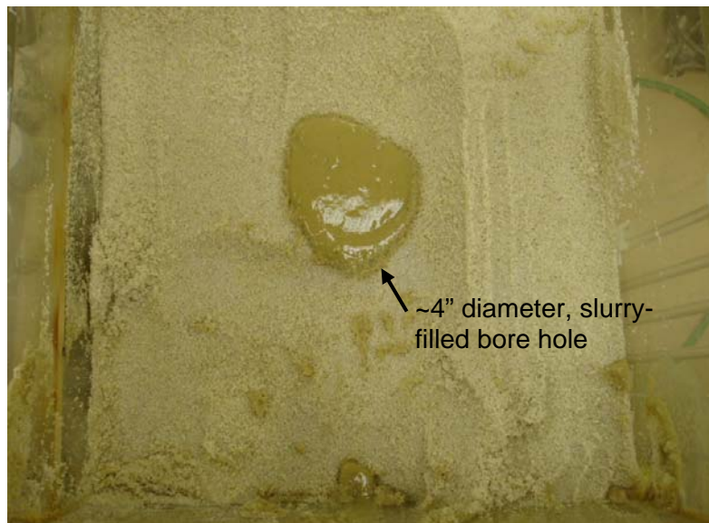
Figure 5. View of excavated sand in liquefaction tank showing the open borehole.
