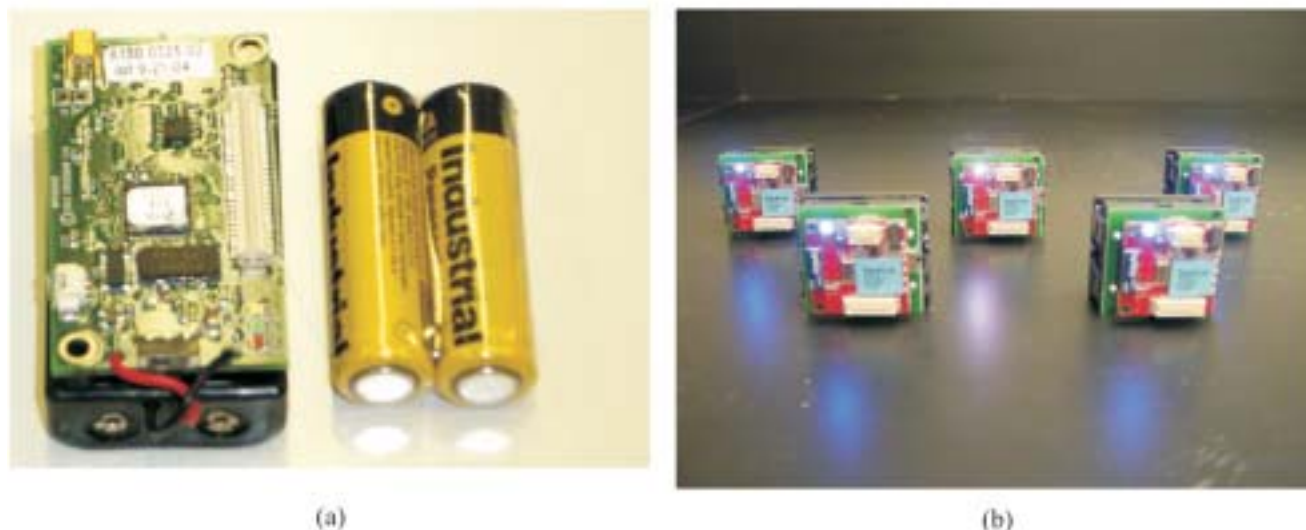
Figure 4. Commercial wireless sensors: (a) Crossbow MICA2 Mote; (b) Intel iMote.
