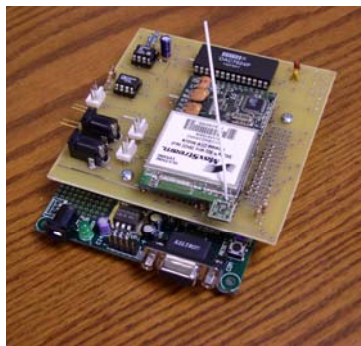
Figure 3 – (Left) wireless active sensing unit prototype, (right) performance specifications
