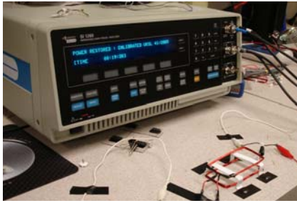
Fig. 8. A Solartron 1260 impedance gain/phase analyzer connected to a coil antenna as the RFID reader.
