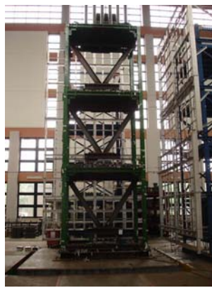
(a) The 3-story test structure
