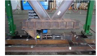
(c) MR damper installed between floors
