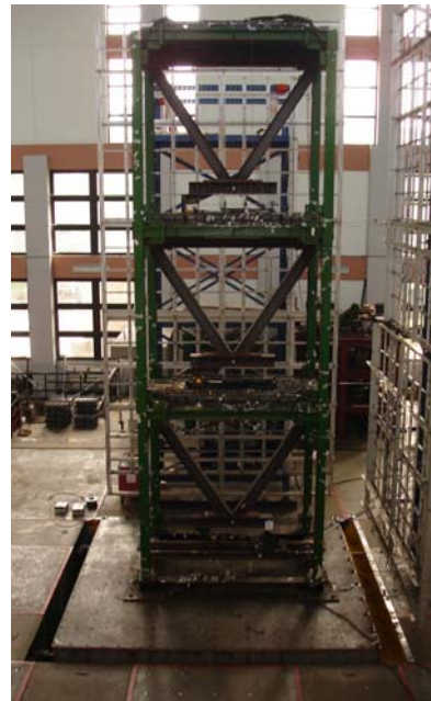
Figure 7. (Left) overview of the wireless control system installed in a 3-story partial scale test structure; (right) the test structure installed upon the NCREE shaking table.
