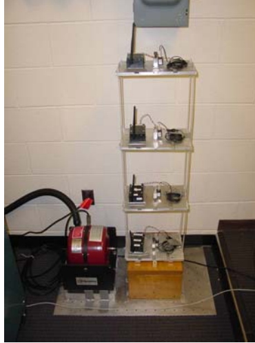
FIGURE 3 – THREE STORY TEST STRUCTURE UPON WHICH WIRELESS SENSORS ARE INSTALLED. MODEL UPDATING IS PERFORMED BY THE WIRELESS SENSOR NETWORK.
