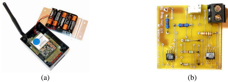
Figure 2. (a) Fully assembled prototype with battery power source revealed, and (b) interface circuit for metal foil strain gages.
