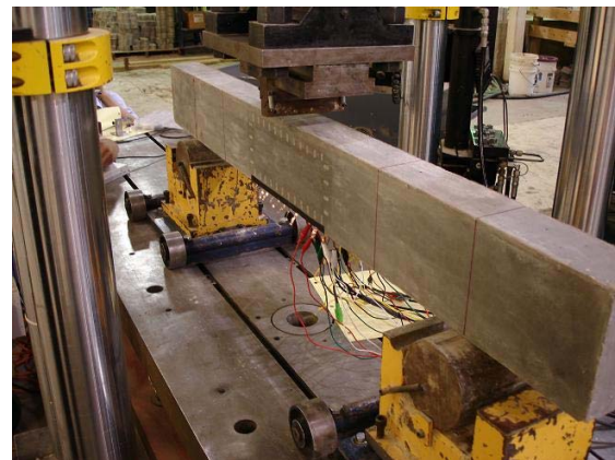
Figure 10. (Left) ECC beam with electrodes applied to lower face. (Right) Experimental setup
