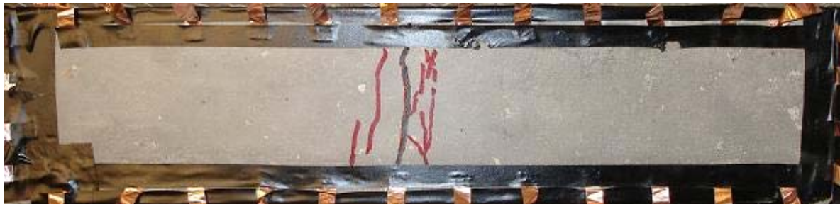
Figure 13. Crack pattern of the ECC beam lower face after damage localization.
