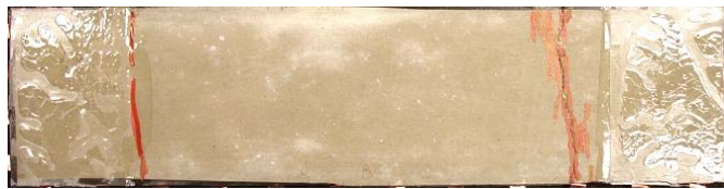
Figure 4. Specimen #1 after monotonic loading is completed and damage has localized in the form of two cracks (denoted with red markings to the left and right sides of the plate).
