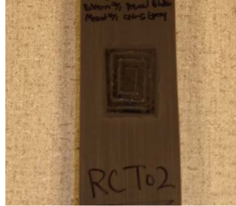
Figure 3: Patterned SWNT-PSS/PVA thin film inductively coupled wireless coil antenna.
