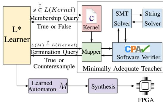
**Figure 2.** AUTOMATASYNTH System Architecture. The MAT uses the legacy kernel to answer membership queries. The mapper combines the kernel and candidate automaton to produce a software verification problem. Using bounded software model checking combined with string decision procedures, we search for a counterexample that distinguishes the target language from the language of the candidate automaton. Finally, we synthesize the learned automaton for execution on an FPGA.
