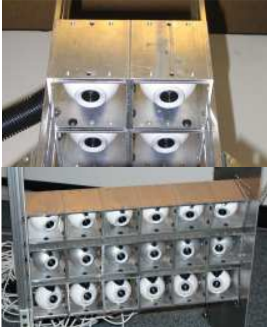
Figure 1: Different configurations of the Reconfigurable Camera Array for Machine Vision Inspection (RAMVI).
