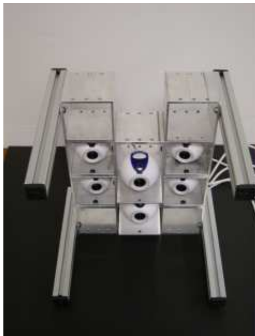
Figure 11: The six-camera RAMVI configuration used in this experiment.
