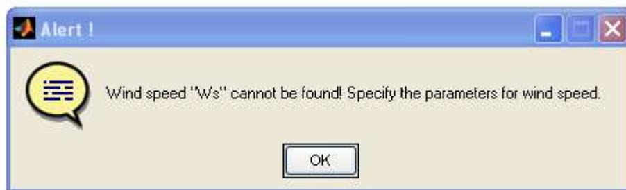
Fig.4. The code is requiring a parameter set for wind speed because it doesn't find such a variable among the inputs.
