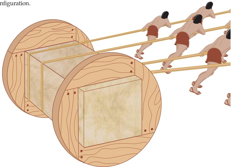
Such removable, wooden devices may, in fact, explain the mysterious "rockers" known from the New Kingdom (1550-1070 B.C.), which some scholars believe were parts of presumed levering machines used to raise the stones. The rockers comprise a pair of thick wooden boards with curved bot-
