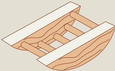
Timbers shaped into rockers have been identified in ancient Egypt. The authors believe such rockers may have been parts or prototypes of rolling devices for pyramid blocks.
