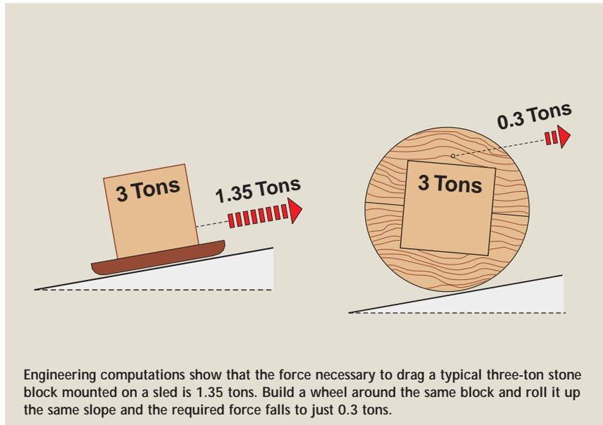
the wheel, but the principle of rolling. A simple assembly of curved wooden parts can create a solid wheel-like device around the block. Mounting such a device near either end of the block would give it an easy-to-roll configuration.
