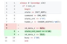
Fig. 3. A representative multi-edit repair by CirFix for a defect in the sdram\_controller benchmark. The original defect, with a missing and an incorrect assignment, is shown in red; the repaired code is shown in green. Edits on lines 8 and 9 correspond to insert and replace operations respectively.
