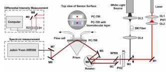
Two detection methods to measure the shift of the resonance mode: a) Spectrum measurement is to measure the shift of the resonance wavelength that provides large detection range (~  $\mu$  m) with a reasonable resolution (~10<sup>-2</sup>nm); b) Differential intensity measurement is used to measure the intensity ratio change of the resonant mode at a single wavelength. This yields a high detection resolution (~10<sup>-5</sup>);
