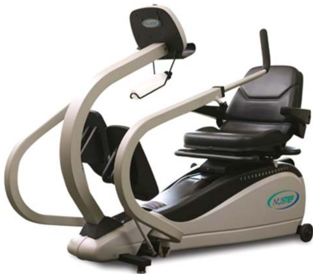
Fig. 1 Recumbent stepping machine (TRS 4000, NuStep, Inc., Ann Arbor, MI). The recumbent stepping machine is driven by pedals and handles that mechanically couple upper and lower limb motion. The left arm and right leg move forward while the right arm and left leg move backward. Both the seat and handles are adjustable to accommodate a full range of motion for participants of different sizes
