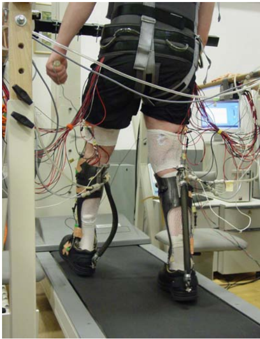
Figure 4. A patient uses bilateral ankle foot orthoses and push button controllers to assist locomotor training.
