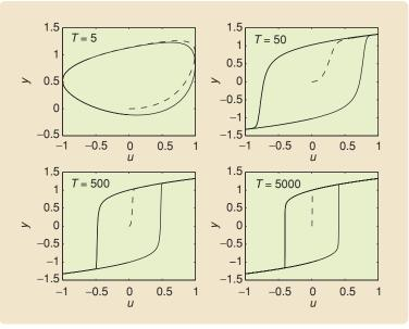
**FIGURE 9** Periodic input-output map  $\mathcal{H}(u_T, x_T(0))$  for the cubic model in Example 4 with  $u_T(t) = \sin(2\pi/T)t$  for several values of T. For each value of T, the transient approach to the periodic input-output map is shown. The system is step convergent, and  $\mathcal{H}(u_T, x_T(0))$  converges to a hysteretic limiting periodic inputoutput map  $\mathcal{H}_{\infty}(u_T, x_0)$  as  $T \to \infty$ , and thus the system is hysteretic.
