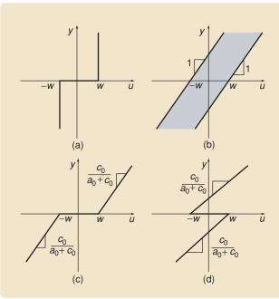
**FIGURE 28** The input-output equilibria map  $\mathcal E$  of (a) case 1 given by (34), (b) case 2 given by (35), (c) case 3 given by (36), and (d) case 4 given by (37). The shape of the input-output equilibria map  $\mathcal E$  determines whether the system is hysteretic or not.
