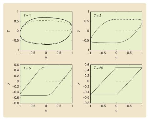
**FIGURE 13** Periodic input-output map for the mass-dashpot-spring system with a deadzone shown in Figure 5, where w=0.5, m=0.1, k=10, c=1, and  $u_T(t)=\sin(2\pi/T)t$  for several values of T. For each value of T, the transient approach to the periodic input-output map is shown. This system exhibits rate-dependent hysteresis because the periodic input-output maps for varying values of T are not identical. The hysteresis map in the lower right is the classical backlash.
