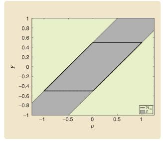
**FIGURE 14** The input-output equilibria map  $\mathcal E$  and the limiting periodic input-output map  $\mathcal H_\infty(u,x_0)$  of the mass/dashpot/spring with deadzone model in Example 6.  $\mathcal H_\infty(u,x_0)$  consists of two horizontal components and parts of the boundary of  $\mathcal E$ .
