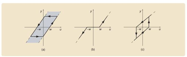
**FIGURE 29** The limiting periodic input-output map  $\mathcal{H}_{\infty}(u, x_0)$  (solid) and the input-output equilibria set  $\mathcal{E}$  (dashed) of (a) case 2, (b) case 3, and (c) case 4 of Figure 28. The input-output maps in (a) and (c) are hysteretic, whereas the map in (b) is not. Furthermore, the hysteretic map in (a) is traversal type, whereas the hysteretic map in (b) is bifurcation type.
