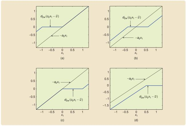
FIGURE 24 The four cases of solutions of (33) with  $a_0 \neq 0$ , and  $a_0 + c_0 = 0$ , and  $c_0 > 0$ . In (a)  $\bar{u} = -w$  and the solutions of (33) form a set  $\mathcal{X} = \{\bar{x} \in \mathbb{R} : \bar{x} \geq 0\}$ ; in (b)  $|\bar{u}| < w$  and  $\mathcal{X} = \{0\}$ ; and in (c)  $\bar{u} = w$  and  $\mathcal{X} = \{\bar{x} \in \mathbb{R} : \bar{x} \leq 0\}$ . Finally, in (d)  $|\bar{u}| > w$  and  $\mathcal{X}$  is empty.
