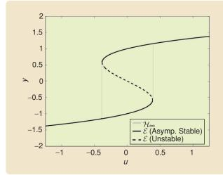
FIGURE 10 The input-output equilibria set  $\mathcal{E}$  and the limiting periodic input-output map  $\mathcal{H}_{\infty}(u, x_0)$  of the cubic model in Example 4.  $\mathcal{E}$  consists of points arising from asymptotically stable (solid) equilibria and from unstable (dashed) equilibria. Note that  $\mathcal{H}_{\infty}(u, x_0) \subseteq \mathcal{E}$  except for the vertical limiting transition trajectories between subsets of  $\mathcal{E}$ .
