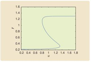
**FIGURE 33** The input-output equilibria map  $\mathcal{E}$  of (39)–(41) with  $\alpha_1=1.3,\ \alpha_2=1.3,\ \beta_1=3,$  and  $\beta_2=6$ . Notice that the shape of  $\mathcal{E}$  given by (39)–(41) is similar to the shape of  $\mathcal{E}$  given by the cubic hysteresis model in Example 4.
