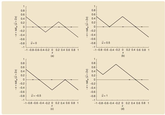
**FIGURE 20** Plots of  $-x + \text{sat}_w(\bar{u} + 2x)$  and the scalar phase portraits of (27) in Example 9, where (a)  $\bar{u} = 0$ , (b)  $\bar{u} = 1/2$ , (c)  $\bar{u} = -1/2$ , and (d)  $\bar{u} = 1$ . The phase portrait analysis shows that (27) is step convergent..
