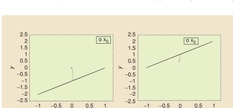
**FIGURE 12** The periodic input-output maps of (24) in Example 5 with  $u(t) = \sin 0.01t$  where (a)  $x_0 = 0$  and (b)  $x_0 = 0.5$ . Note that (24) is not hysteretic although  $\mathcal{E}$  of (24) is a multivalued map as shown in Figure 11.
