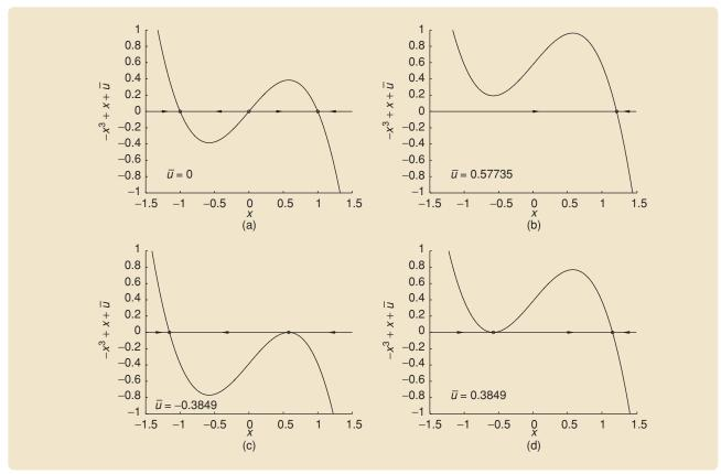
FIGURE 17 Plots of  $-x^3 + x + \overline{u}$  and the phase portraits of (19), where (a)  $\overline{u} = 0$ , (b)  $\overline{u} = -(2/3\sqrt{3})$ , (c)  $\overline{u} = (2/3\sqrt{3})$ , and (d)  $\overline{u} = (1/\sqrt{3})$ . The phase portrait analysis shows that (19) is step convergent.
