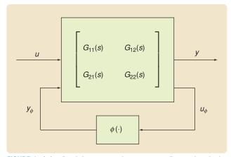
**FIGURE 1** A feedback interconnection corresponding to the single-input, single-output system (1)–(4). The interconnection involves a two-input/two-output linear system and a feedback nonlinearity. Note that the model can be interpreted as the linear fractional transformation between the nonlinearity  $\phi(\cdot)$  and  $G_{11}$ ,  $G_{12}$ ,  $G_{21}$ , and  $G_{22}$ .
