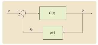
**FIGURE 2** Feedback interconnection of the nonlinear hysteresis model (7), (8), where  $G(s) \stackrel{\triangle}{=} C(sI-A)^{-1}B$ . This model is a simplification of the nonlinear feedback model in Figure 1 obtained by setting D=B,  $E_0=0$ ,  $E_1=C$ , that is, with  $G_{11}=G_{12}=G_{21}=G_{22}=G(s)$ .
