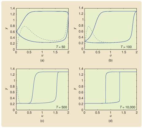
FIGURE 35 The periodic input-output map  $\mathcal{H}(u_T, x_T(0))$  corresponding to (39)-(41) with  $u_T(t) = 2|\sin(2\pi/T)t|$ . Note that  $\mathcal{H}(u_T, x_T(0))$  converges to a hysteretic map  $\mathcal{H}_{\infty}(u, x_0)$  as
