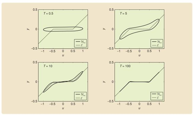
FIGURE 30 Periodic input-output map  $\mathcal{H}(u_T, x_T(0))$  and input-output equilibria map  $\mathcal{E}$  of Example 11 with  $u(t) = \sin(2\pi/T)t$ . Note that this model is case 3 and is not hysteretic.
