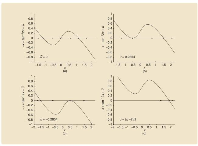
FIGURE 18 Plots of  $-x + \bar{u} + \tan^{-1} 2x$  and the phase portraits of (26) in Example 8, where (a)  $\bar{u} = 0$ , (b)  $\bar{u} = (\pi - 2)/4$ , (c)  $\bar{u} = -(\pi - 2)/4$ , and (d)  $\bar{u} = (\pi - 2)/2$ . The phase portrait analysis shows that (26) is step convergent.
