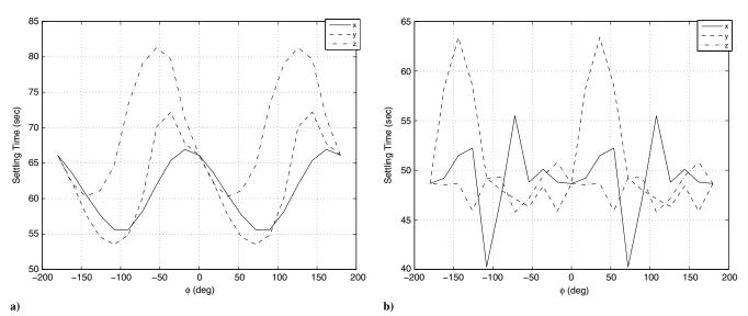
Fig. 8 Settling time as a function of principal-frame/body-frame rotation angle  $\phi$  for rotations about each of the three principal axes of  $J_3$ . Convergence is achieved for a) control law (44) and b) control law (53).
