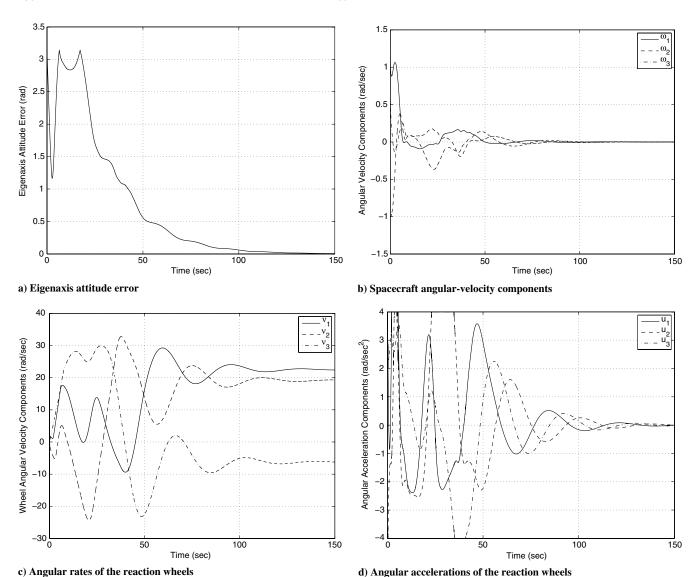
Fig. 3 Slew maneuver using the control law (44) with no disturbance. The acceleration of the reaction wheels is saturated at 4 rad/s<sup>2</sup>.
