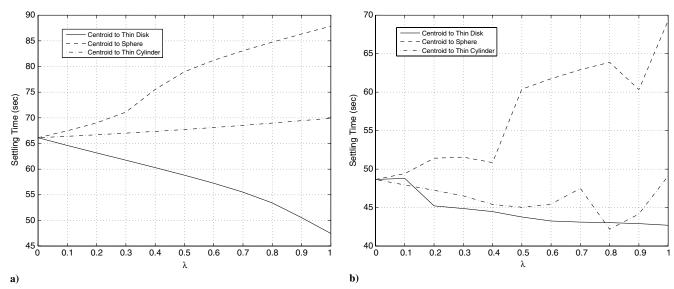
Fig. 7 Settling time as a function of  $\lambda$  for various combinations (41) of inertia matrices resolved in principal frames. Convergence is achieved for a) control law (44) and b) control law (53). Each controller is implemented in all cases with a single tuning. In all cases, the bus inertia  $J_3$  is unknown.
