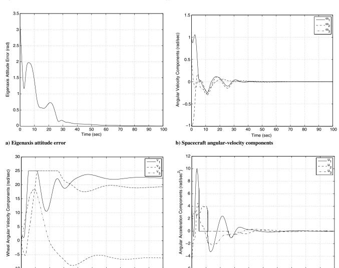
Fig. 5 Slew maneuver using the control law (44) with no disturbance. The maximum rotation rate of each wheel is saturated at 25 rad/s.
