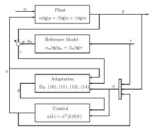
Fig. 1 Schematic diagram of the RC-MRAC architecture given by Eqs. (6), (13), and (14).
