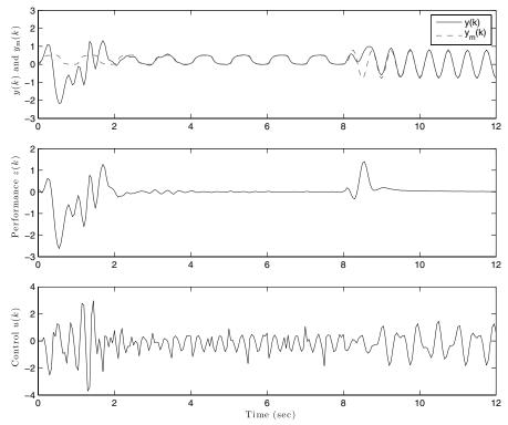
Fig. 11 Sampled-data, three-mass structure. The RC-MRAC algorithm (6), (13), and (14) is implemented in feedback with  $n_c = 16$ ,  $\lambda = 1$ ,  $P(0) = 10^2 I_{2n_c+1}$ , and  $\theta(0) = 0$ . The adaptive controller forces *z* asymptotically to zero; thus, the position of  $m_3$  follows  $y_m$  while rejecting *w*. Note that *y* continues to follow the command  $y_m$  after 8 s when *r* is changes to a 2 Hz sinusoid.
