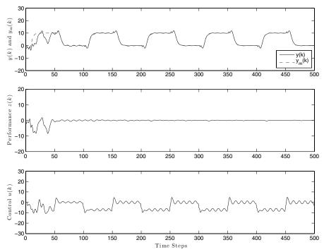
Fig. 5 Lyapunov-stable, nonminimum-phase plant with disturbance. The RC-MRAC algorithm (6), (13), and (14) is implemented in feedback with  $n_c = 10$ ,  $\lambda = 1$ ,  $P(0) = I_{2n_c+1}$ , and  $\theta(0) = 0$ . The adaptive controller drives *z* to zero. Thus, *y* follows  $y_m$  while rejecting *w*.
