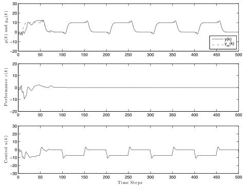
Fig. 4 Lyapunov-stable, nonminimum-phase plant without disturbance. The RC-MRAC algorithm (6), (13), and (14) is implemented in feedback with  $n_c = 40$ ,  $\lambda = 1$ ,  $P(0) = I_{2n-1}$ , and  $\theta(0) = 0$ . The closed-loop performance is comparable to that shown in Fig. 3.
