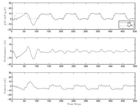
Fig. 6 Lyapunov-stable, nonminimum-phase plant with disturbance and 10% error in the estimates of the nonminimum-phase zeros. The RC-MRAC algorithm (6), (13), and (14) is implemented in feedback with  $n_c = 10$ ,  $\lambda = 1$ ,  $P(0) = I_{2n_c+1}$ , and  $\theta(0) = 0$ . The adaptive controller yields over 70% improvement in the performance *z* relative to the open-loop performance.
