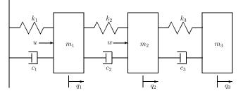
Fig. 10 A serially connected three-mass structure subjected to disturbance w and control u.
