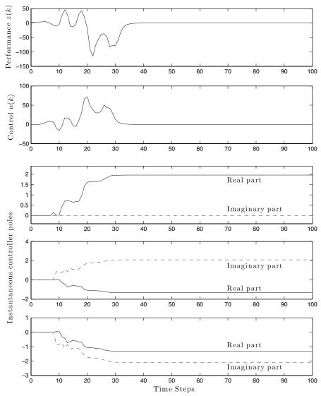
Fig. 7 Stabilization of a plant that is not strongly stabilizable. The RC-MRAC algorithm (6), (13), and (14) is implemented in feedback with  $n_c = 3$ ,  $\lambda = 1$ ,  $P(0) = I_{2n_c+1}$ , and  $\theta(0) = 0$ . The adaptive controller forces *z* asymptotically to zero, thus stabilizing the plant, which is not strongly stabilizable.
