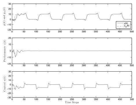
Fig. 3 Lyapunov-stable, nonminimum-phase plant without disturbance. The RC-MRAC algorithm (6), (13), and (14) is implemented in feedback with  $n_c = 10$ ,  $\lambda = 1$ ,  $P(0) = I_{2n_c+1}$ , and  $\theta(0) = 0$ . The adaptive controller drives *z* to zero.
