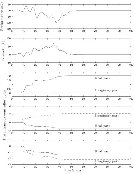
Fig. 8 Stabilization of a plant that is not strongly stabilizable with error in the estimate of the nonminimum-phase zero. The RC-MRAC algorithm (6), (13), and (14) is implemented in feedback with  $n_c = 3$ ,  $\lambda = 1$ ,  $P(0) = I_{2n_c+1}$ , and  $\theta(0) = 0$ . The plant's nonminimum-phase zero is located at 1.1, and RC-MRAC uses an estimate of the nonminimum-phase zero given by 1.04. The adaptive controller stabilizes the plant, which is not strongly stabilizable.
