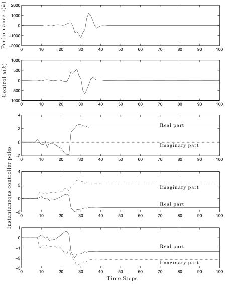
Fig. 9 Stabilization of a plant that is not strongly stabilizable with error in the estimate of the nonminimum-phase zero. The RC-MRAC algorithm (6), (13), and (14) is implemented in feedback with  $n_c = 3$ ,  $\lambda = 1$ ,  $P(0) = I_{2n_c+1}$ , and  $\theta(0) = 0$ . The plant's nonminimum-phase zero is located at 1.1, and RC-MRAC uses an estimate of the nonminimum-phase zero given by 1.199. The adaptive controller stabilizes the plant, which is not strongly stabilizable.
