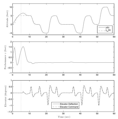
Fig. 12 NASA's GTM. The RC-MRAC algorithm (6), (13), and (14) is implemented in feedback with  $n_c = 20$ ,  $\lambda = 1$ , and  $P(0) = 10^{20}I_{2n_c+1}$ . The adaptive controller force the aircraft's altitude *y* to follow the reference model  $y_m$ .
