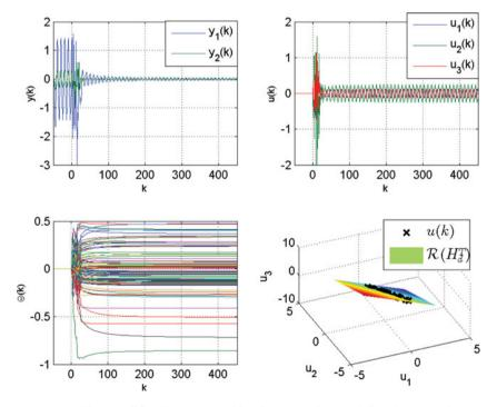
Figure 13. Example 4.2, RCAC with  $\eta$ -modification: We consider the same plant and disturbance as in Example 4.2, and apply the cumulative update law with  $\eta$ -modification. We use  $n_c = 6$ ,  $P_0 = I$ ,  $\eta_0 = 0.1$ , and  $\eta_1 = 0.05$ . Despite the unmodelled NMP input-subspace zero,  $\Theta$  converges, y is driven towards zero, and u is bounded.
