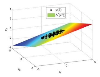
Figure 12. This figure illustrates the phase portrait for  $k \in [800, 1000]$  of the output *y* for Example 4.4 shown in Figure 6. Since the output-subspace zeros of  $G_{yu}$  are minimum phase, the performance output *y* is bounded, and oscillates on the surface  $\mathcal{N}(H_1^T)$ . Since *y* is contained in  $\mathcal{N}(H_1^T)$ , the controller  $\Theta$  converges.
