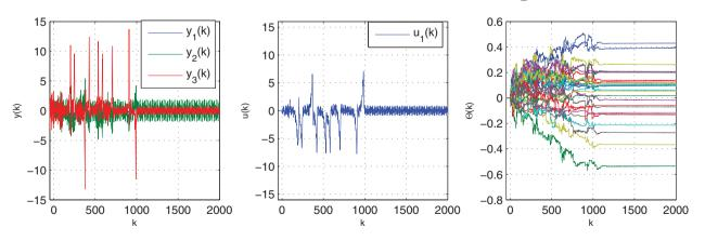
Figure 15. Example 4.5, RCAC with  $\eta$ -modification: We consider the same plant and disturbance as in Example 4.5, and apply the instantaneous update law with  $\eta$ -modification. We use  $n_c = 7$ ,  $\mu = 20$ ,  $\eta_0 = 0$ , and  $\eta_1 = 0.01$ . Despite the unmodelled NMP output-subspace zero,  $\Theta$  converges, and u and y are bounded.
