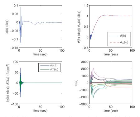
Figure 16. Boeing 747 longitudinal dynamics: We apply RCAC without  $\eta$ -modification. Although the pitch angle follows the output of the reference model, the elevator deflection and thrust excursion oscillate during the transient with peak magnitudes 71 deg and 36 ft/sec<sup>2</sup>, respectively. The control inputs are not within practical saturation limits.
