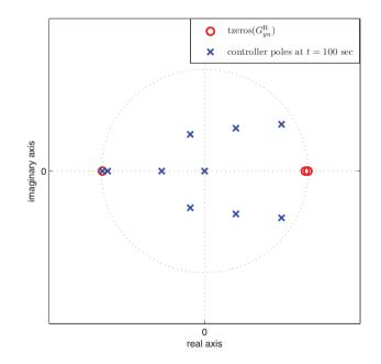
Figure 17. This figure illustrates the input-subspace zeros of the Boeing 747 longitudinal dynamics along with the poles of the adaptive controller at t = 100 sec. The adaptive controller places a pole near the input-subspace zero -0.9857. This polezero cancellation near the unit circle causes large transients in the elevator deflection and thrust excursion, as illustrated in Figure 16.
