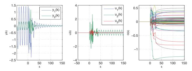
Figure 2. Example 4.1: unmatched disturbance rejection for the minimum-phase,  $2 \times 3$  wide plant (38) and (39). The performance output *y* approaches zero, the control signal *u* is bounded, and the controller  $\Theta$  converges.
