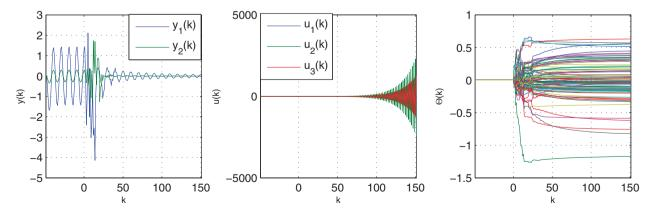
Figure 3. Example 4.2: unmatched disturbance rejection for the 2 × 3 wide plant (38) and (39) except that  $B_{(1,1)} = -1.8$ . Although  $G_{yu}$  is minimum phase, the control signal *u* grows without bound, while the performance output *y* approaches zero. The controller  $\Theta$  converges.
