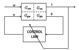
Figure 1. Adaptive output feedback control architecture.
