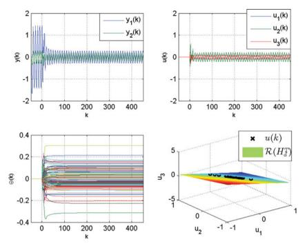
Figure 14. Example 4.2, RCAC with  $\eta$ -modification: Increasing the constant penalty term  $\eta_0$  to 1 leads to a reduction in the control effort as well as a degradation in the steady-state performance level. Thus,  $\eta$ -modification introduces a trade-off between control effort and steady-state performance.
