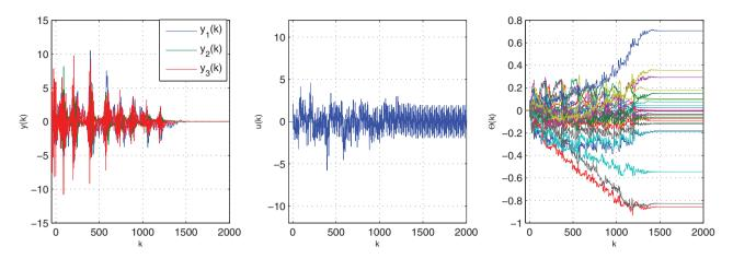
Figure 4. Example 4.3: Matched disturbance rejection for the minimum phase,  $3 \times 1$  tall plant (40) and (41). The controller  $\Theta$  converges, *u* is bounded, and *y* asymptotically approaches zero. RCAC cancels the matched sinusoidal disturbance from three outputs using only one actuator.
