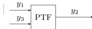
Figure 5. The signals y_1 and y_3 are the inputs and y_2 is the output of the 2ISO PTF.
