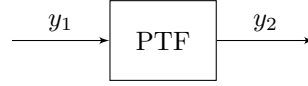
Figure 4. Definition of the PTF. The PTF is a linear system whose input and output are the linear system outputs y_1 and y_2 , respectively. These signals are the pseudo-input and pseudo-output, respectively.
