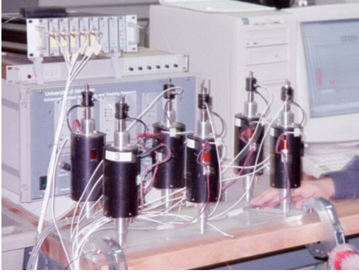
Figure 2: The strut identification test jig
