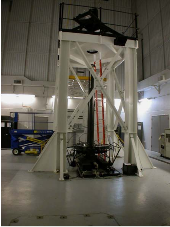
Fig. 2. The metrology tower for the DOT testbed.
