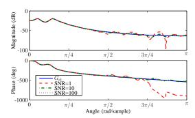
Fig. 5. As the SNR increases, the frequency response of  $\hat{G}_{\rm cl}$  more closely approximates the frequency response of  $G_{\rm cl}$ .
