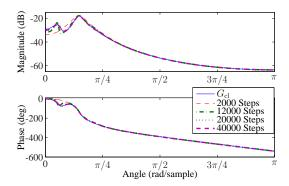
Fig. 6. As the amount of data increases, the frequency response of  $\hat{G}_{\rm cl}$  more closely approximates the frequency response of  $G_{\rm cl}$ .
