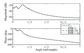
Fig. 8. As the SNR increases, the frequency response of  $\hat{G}_{\rm cl}$  more closely approximates the frequency response of  $G_{\rm cl}$ .
