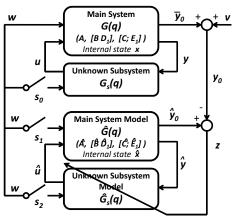
Fig. 1. Model-refinement architectures. The switches  $s_0$ ,  $s_1$  and  $s_2$  are used to define different architectures.
