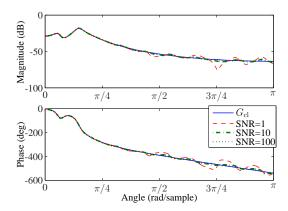
Fig. 4. As the SNR increases, the accuracy of the frequency response of  $\hat{G}_{\rm cl}$  improves.
