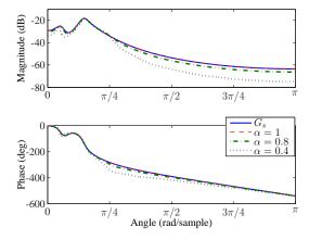
Fig. 10. Estimate of  $G_{\rm cl}$  with uncertain  $\hat{c}_2 = \alpha c_2$ . As  $\alpha$  approaches 1, the frequency response of  $\hat{G}_{\rm cl}$  more closely approximates the frequency response of  $G_{\rm cl}$ .
