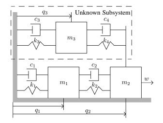
Fig. 2. Spring-mass-damper system with main system and unknown subsystem.
