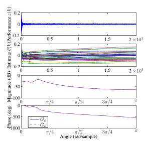
Fig. 3. The RCO algorithm is turned on at k=100 steps. The closed-loop frequency response of  $\hat{G}_{\rm cl}$  is indistinguishable from the frequency response of  $G_{\rm cl}$ .
