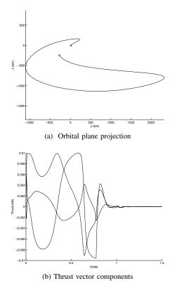
Fig. 3: Rendezvous maneuver performed at perigee on a Molniya orbit with 10 N saturated thrust. (a) Orbital plane projection; (b) Thrust vector components.
