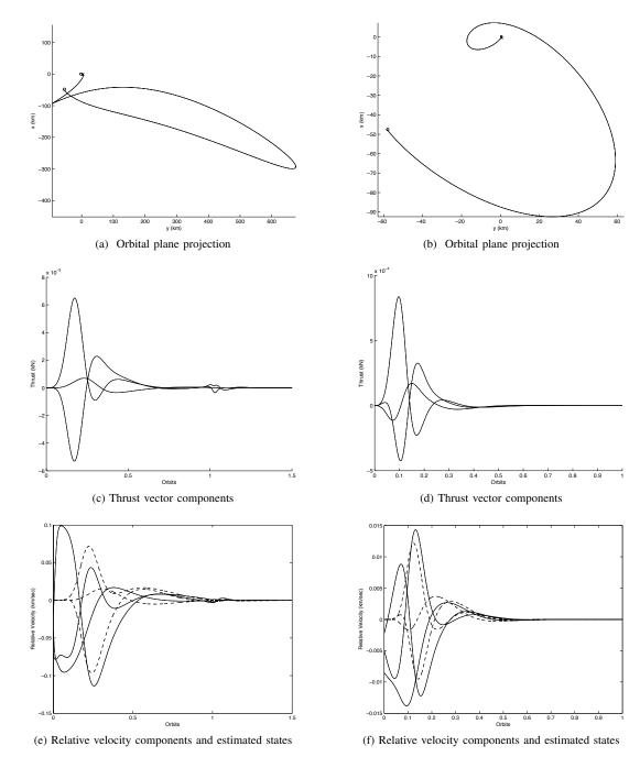
Fig. 9: Output feedback rendezvous maneuver performed at perigee on Molniya (left) and Tundra (right) orbits with 10-N saturated thrust. Only relative position data is assumed to be available. (a),(b) Orbital plane projection; (c),(d) Thrust vector components; (e),(f) Relative velocity components and estimated states.
