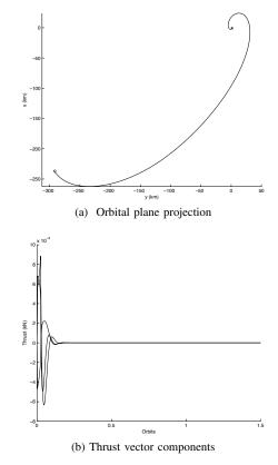
Fig. 4: Rendezvous maneuver performed at perigee on a Tundra orbit with 10 N saturated thrust. (a) Orbital plane projection; (b) Thrust vector components.
