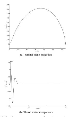
Fig. 6: Rendezvous maneuver performed at perigee on a Tundra orbit with 10 N saturated thrust aligned with the ram direction. (a) Orbital plane projection; (b) Thrust vector components.
