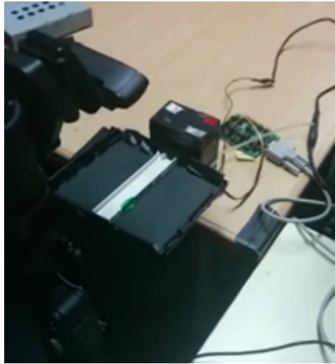
Figure 7.3: The ball balancing experimental setup for the reduced 1D case.
