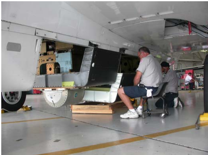
Figure 2. PSR undergoing installation on the WB-57.
