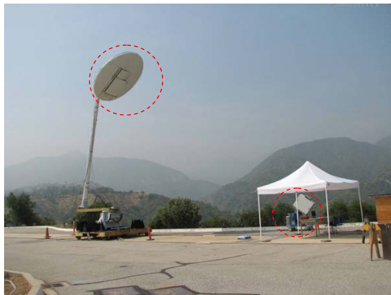
Figure 4.2: Experimental Setup at the JPL Mesa Outdoor Antenna Range. The Earth disk target is highlighted in the upper left and GeoSTAR-D in the bottom right.
