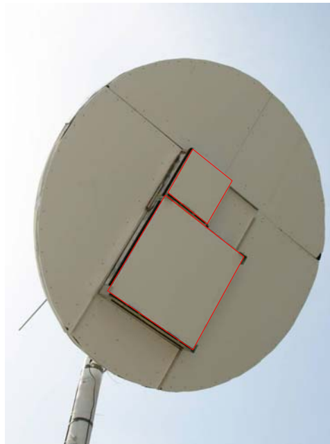
Figure 4.4: Earth Disk Target with the Two Independent Heating Zones Highlighted in Red
