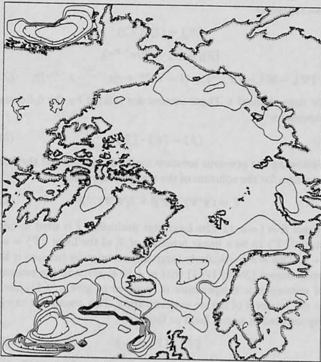
Fig. 7. Atmospheric water vapor contours as derived from the weather-correcting algorithm over the Arctic for October 4, 1978. The contours represent 1, 2, 3 (hatched lines) and 4 \text{g/cm}^2 of integrated water vapor. The high concentration of water vapor in the North Atlantic Ocean and the Gulf of Alaska correlate with the false retrievals of sea ice shown in Figure 5. The false retrievals in the Bering Sea are a result of high winds in the area.
