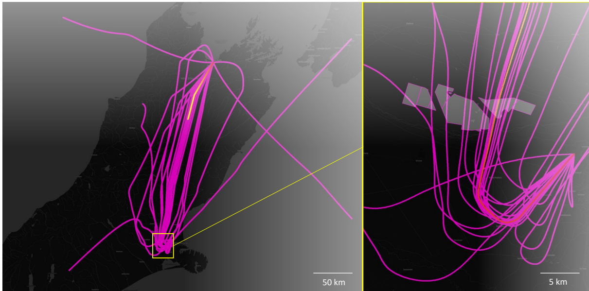
Fig. 4. Example flight from Christchurch to Nelson. Left: pink lines represent the location of reflected GNSS signals during the flight (flight direction: south to north). Right: inset map illustrating representative data for a farm near Christchurch airport.
