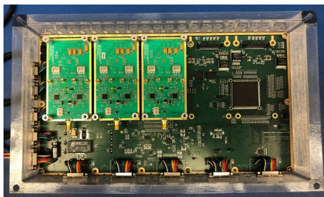
Figure 4. Next generation GNSS-R receiver shown with three RF front end daughter boards installed.
