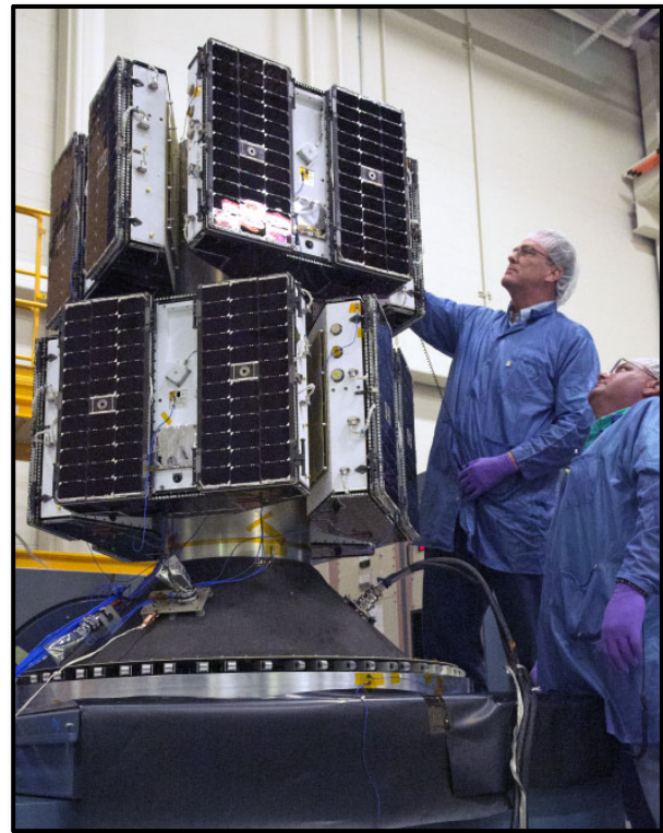
Figure 1. The eight CYGNSS observatories in the “flight stack” configuration, mounted concentrically around a central deployment module, undergoing vibration testing.
