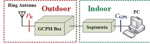
Fig. 1. The measurement setup of the GCPM system
