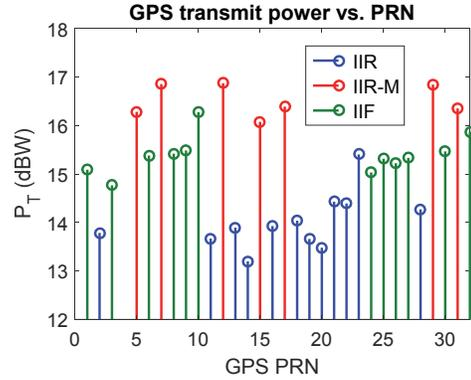
Fig. 5. Estimated GPS transmit power  $P_T$  vs. GPS PRN
