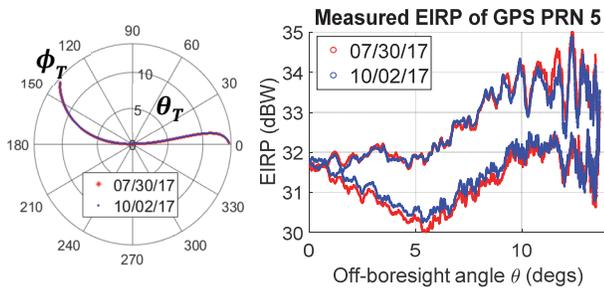
Fig. 7. Cuts through the pattern and GCPM's measured EIRPs
