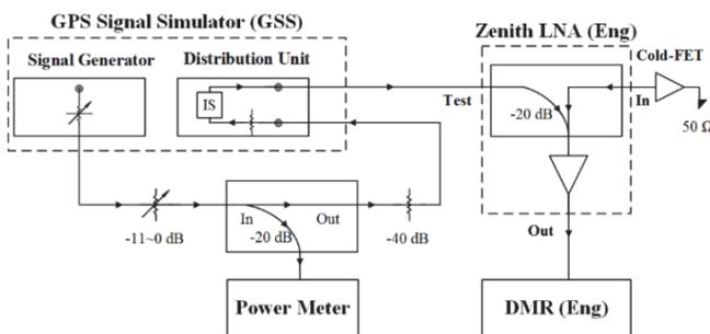
Fig. 9. Calibration scheme of CYGNSS zenith measurement
