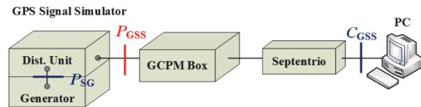
Fig. 2. Single PRN calibration using GSS
