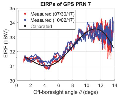
Fig. 6. Measured and calibrated EIRPs
