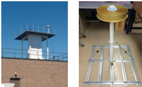
(a). Location (b). Side view Fig. 4. Javad RingAnt-DM antenna
