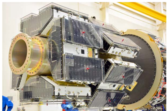
Fig 1. The "flight stack" of eight observatories are shown concentrically mounted around the central cylindrical deployment module, which is attached to the third stage of the launch vehicle by a tapered adapter cone.
