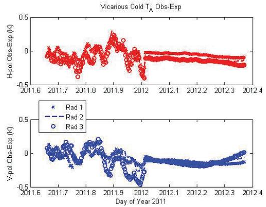
**Figure 6.** Vicarious cold bias estimate (Obs-Exp) oceanic RFI-free  $T_{AS}$ , including V1.3 and V1.3-DR data.
