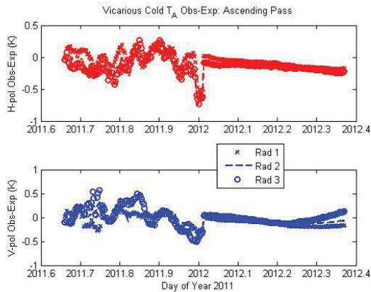
**Figure 9.** Vicarious cold bias estimate (Obs-Exp) for ascending pass oceanic RFI-free  $T_{AS}$ .
