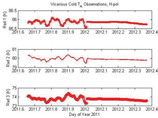
**Figure 3.** Vicarious cold statistic for RFI-free oceanic H-pol  $T_{AS}$ , including V1.3 and V1.3-DR data.
