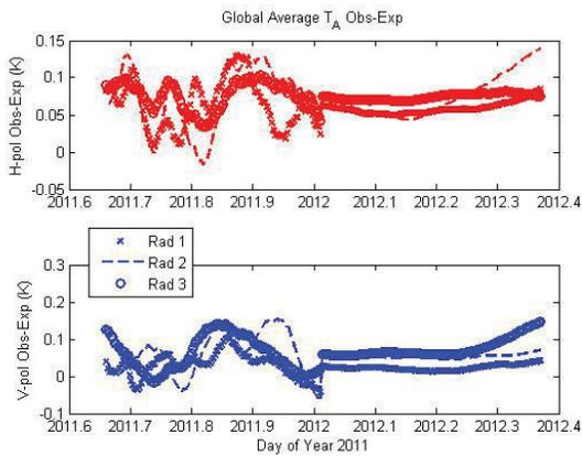
**Figure 5.** Global average bias estimate (Obs-Exp) oceanic RFI-free  $T_{AS}$ , including V1.3 and V1.3-DR data.
