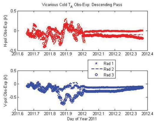
**Figure 10.** Vicarious cold bias estimate (Obs-Exp) for descending pass oceanic RFI-free  $T_{AS}$ .
