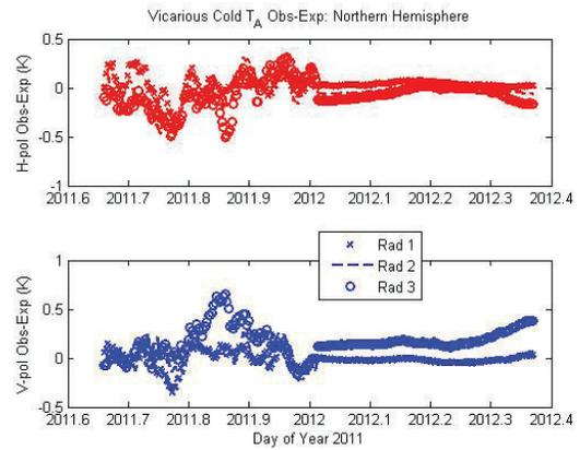
**Figure 7.** Vicarious cold bias estimate (Obs-Exp) for Northern Hemisphere oceanic RFI-free  $T_{AS}$ .
