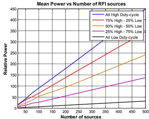
Fig. 6. Mean value of relative RFI power vs. increasing number of RFI sources. Different curves represent different fractions of low duty-cycle sources present in the RFI signal
