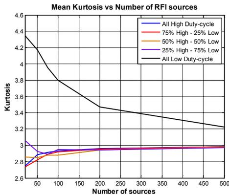
Fig. 5. Mean value of kurtosis vs. increasing number of RFI sources. Different curves represent different fractions of low duty-cycle sources present in the RFI signal
