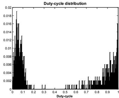
Fig. 3. Bimodal distribution applied for duty-cycle of individual RFI sources, the fraction of low duty-cycle to high duty-cycle is a variable parameter
