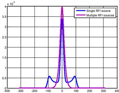
Fig. 4. Probability distribution of RFI with thermal noise (blue-single source, purple-multiple sources)
