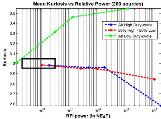
Fig. 7. Mean value of kurtosis vs. RFI power (in NEDT) for 200 sources. (Blue – All high  $d$ , Red – 50%  $d$ , Green – All low  $d$ , Black rectangle – Undetectable problematic RFI)
