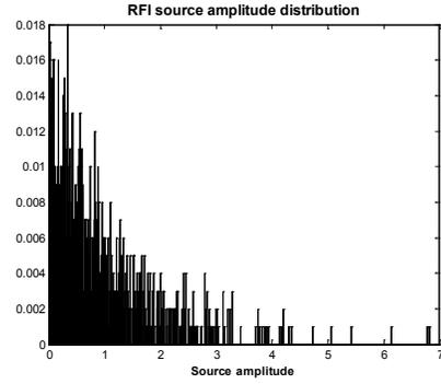
Fig. 2. Exponential distribution applied for amplitude of individual RFI sources, the mean of the exponential distribution is a variable parameter
