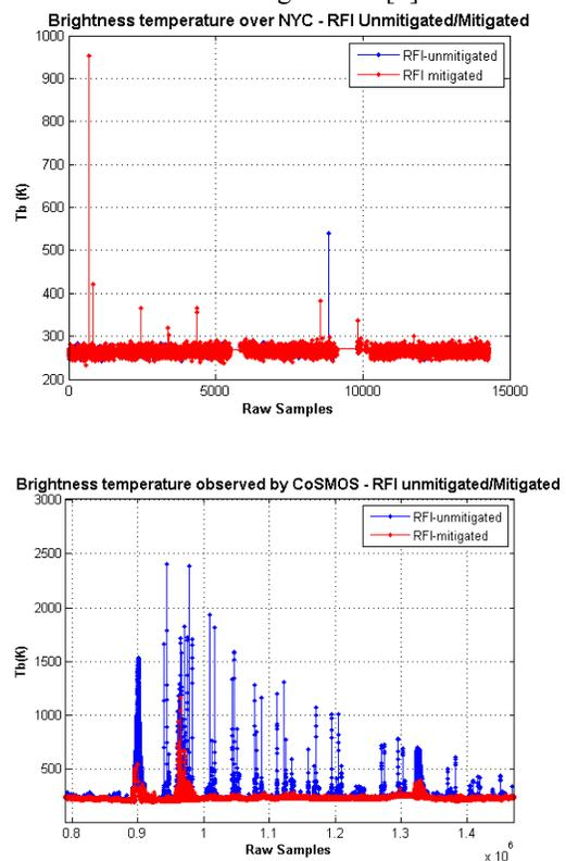
Fig. 1. Brightness temperature values over (a) New-York and (b) Central Europe indicating RFI (blue-unmitigated  $T_b$ , red-RFI mitigated  $T_b$  using full-band kurtosis)
