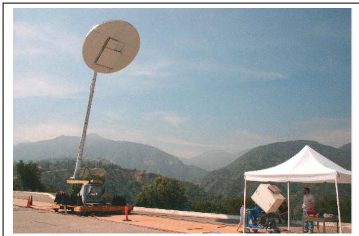
Figure 1. GeoSTAR test setup. GeoSTAR is the white box to the right, which tilted up by about 39 degrees. The target disk is at a range of 16 meters to the west. The 2x2 and 4x4 heated boxes inside of the disk are visible.
