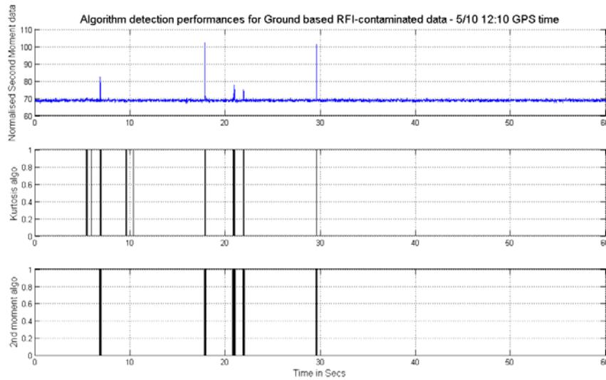
Figure 1. RFI detection of PALS-ADD L-Band radiometer measurements of nadir sky view with strong RFI present: (top) 2<sup>nd</sup> moment time series; (center) kurtosis of signal shows all RFI present; (bottom) Aquarius RFI detection algorithm catches most but not all RFI.
