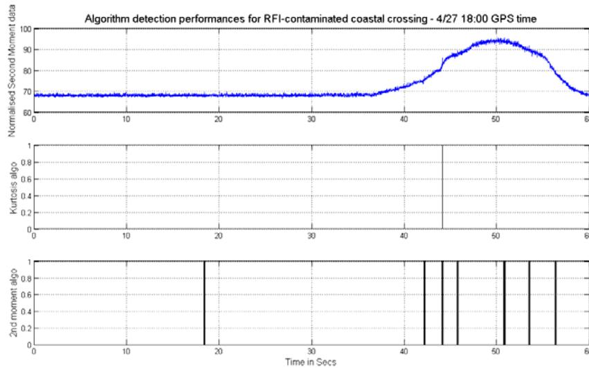
Figure 3. Similar to Fig. 2 but with a single RFI event artificially added at the point of maximum time-rate-of-change of TB during simulated coastal crossing. (top) 2<sup>nd</sup> moment time series; (center) kurtosis of signal detects single RFI event; (bottom) Aquarius RFI detection algorithm detects the true RFI event as well as the false alarms.
