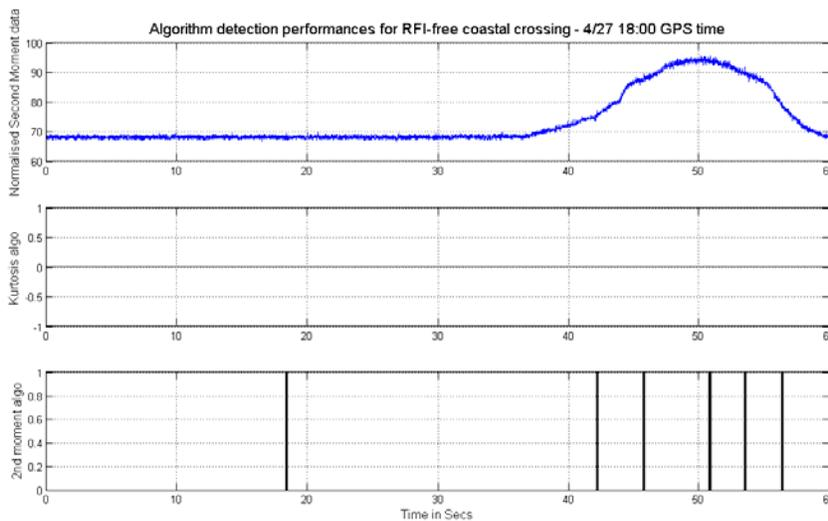
Figure 2. PALS-ADD L-Band radiometer measurements during transition from nadir sky view to BB absorber. Rate of change of TB during transition matches that of Aquarius radiometer during coastal crossing. (top) 2<sup>nd</sup> moment time series; (center) kurtosis of signal shows no RFI present; (bottom) Aquarius RFI detection algorithm has some false alarm – they are more likely when the TB is changing quickest.
