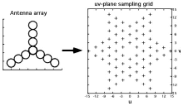
Fig. 3. Antenna array and UV samples
