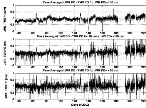
Figure 1. Pass averaged JMR – TMR path delays for low, medium, and high PD bins shown for JMR cycles 3 – 20.
