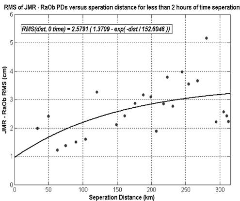
Figure 2. RMS error between the JMR and RaOb Path Delays as a function of spatial separation for measurements with less than 2 hours of time separation.
