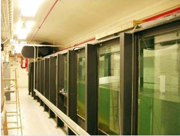
Figure 43: Downwind view of the wind-wave tank from. The suction fan providing the wind forcing can be seen at the end.
