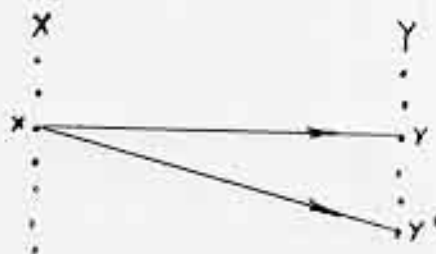
Figure II.1 This is a transformation—two distinct letters ( x and x' ) can be posted to the same address ( y ). (Many-one map).
