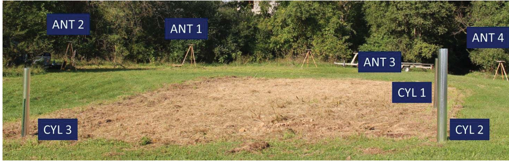
Fig. 2. Change experiment using a four-element multistatic array (Ant 1–4). Three cylinders (Cyl 1–3) were added and removed from the scene.
