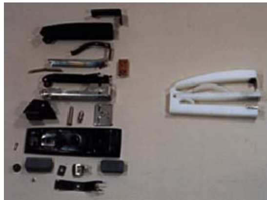
Figure 1-3: A compliant stapler significantly reduces the number of parts in a traditional stapler (Ananthasuresh and Saggere, 1994).
