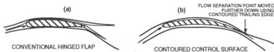
Figure 1-11: (a) A hinged flap that leads to earlier flow separation; (b) a smooth, continuous surface with improved aerodynamic characteristics.
