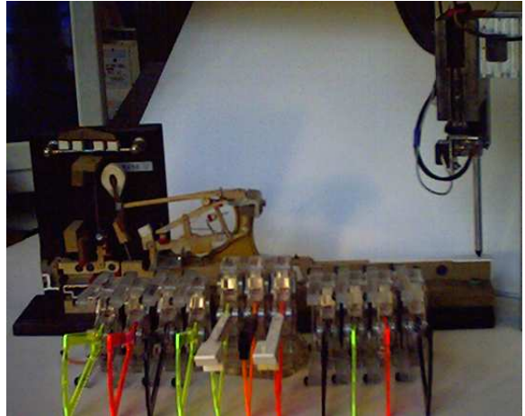
Figure 1. On the right a motorized instrumented probe presses on a piano key. In the foreground a prototype force reflecting synthesizer keyboard is visible.
