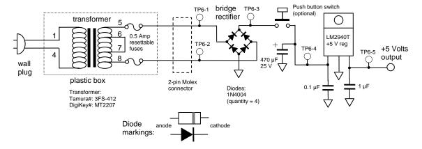
Put a small wire loop at each of the test points (TP6-X).
