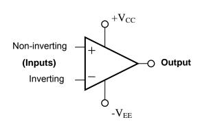
for op-amps to be supplied on a single integrated circuit chip, with either one, two, or four op-amps on a single IC, where each op-amp cam be operated independently. Each op-amp has two inputs and one output. The inputs are designated inverting (-) and non-inverting (+). The figure can be drawn with either input on top, so it is necessary to label the inputs accordingly (+ or -)
